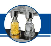
The CVC SC202 is equipped with two bottle nozzles for continuous counting and filling. One bottle is always in place for filling. The operator simply picks up a full bottle and replaces it with an empty bottle.
